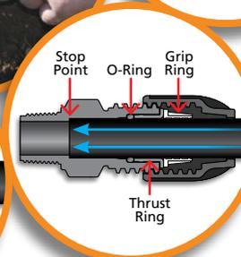
3. Insert the pipe into the fitting through the Nut, White Grip Ring & Thrust Ring until it meets resistance at the O-Ring. Give the pipe a firm push past the O-Ring all the way until it hits the final stop point.
